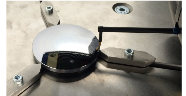
Part photo on Taylor Hobson Form Talysurf
